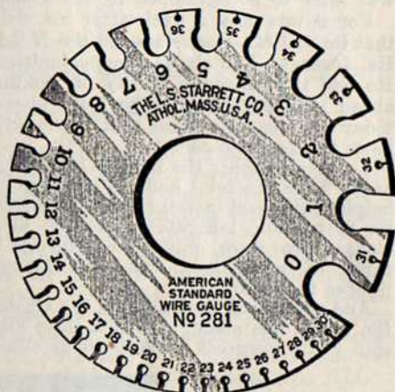
Fig. 1—A Pocket Wire Gauge which can be purchased from any hardware store handling copper wire.
